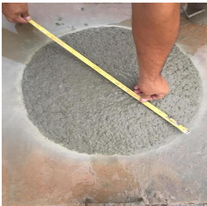
Figura 4.2.4.3 – Teste de Slump/Flow
