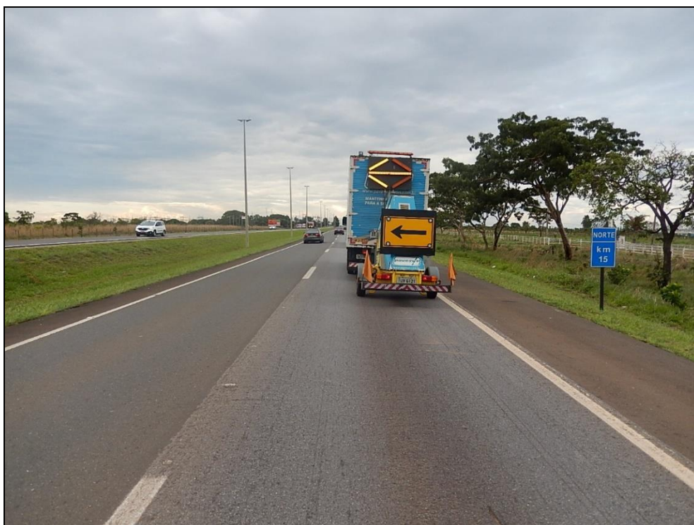
Figura 2.28: Falling Weight Deflectometer Pavesys (FWD)
