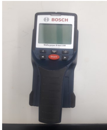
Figura 3.9 – Pacometro Bosch Wallscanner D-tect 150
