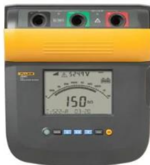
Figura 4.3 – Megômetro digital FLUKE (FLUKE, 2010)
