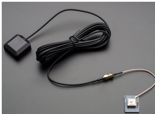
Figura 3.7 – Antena GPS externa 3-5V, 28dB, conectada ao receptor [ADAFRUIT INDUSTRIES, 2022].
