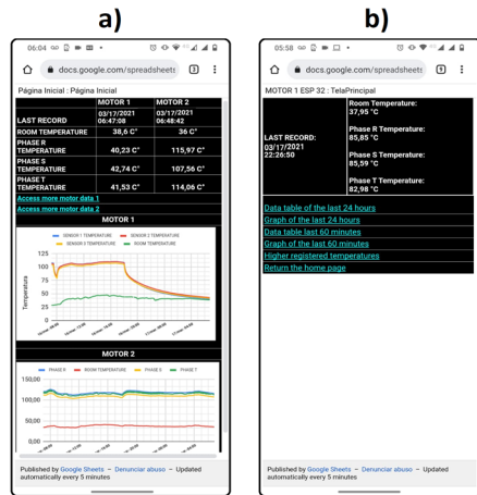
Figure 5: Application screen viewed by a browser on an Android device: (a) Application Home page, shows latest sensor readings and graphs for the last 24 hours and (b) exclusive page to access Motor 1's data.
